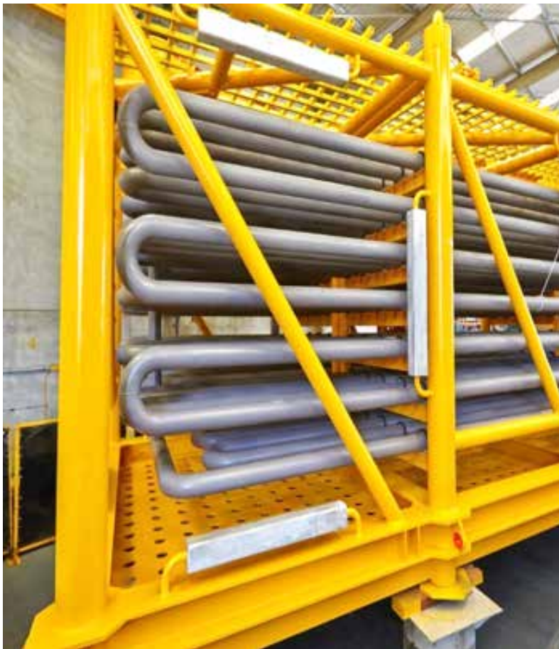
Subsea passiv cooler
